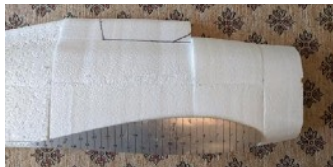
Cockpit area with wing root template in place and cockpit cutout marked.
