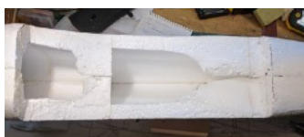
Bottom view of the wing mounting area after the cut out. Lots of room to put stuff in there.
