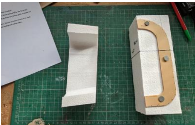
Fuselage section F2 to F3, one side cut, the other side still a blank with the formers nailed on and ready to cut.
