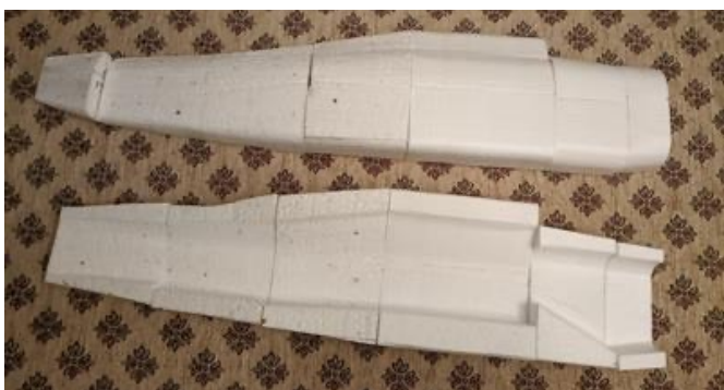
Fuselage section F2 to F3, one side cut, the other side still a blank with the formers nailed on and ready to cut.
