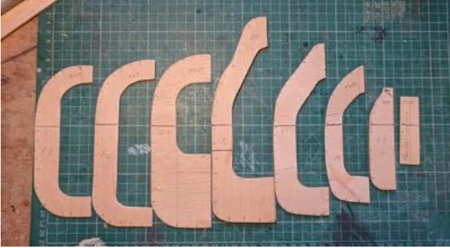
The formers, all marked with the central datum line
