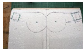
Centre sections glued together with the retracts positions marked
