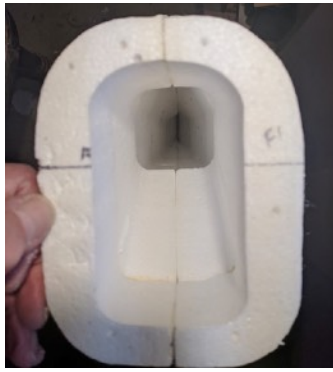
Sections stuck together – inside view looking down towards the tail.
