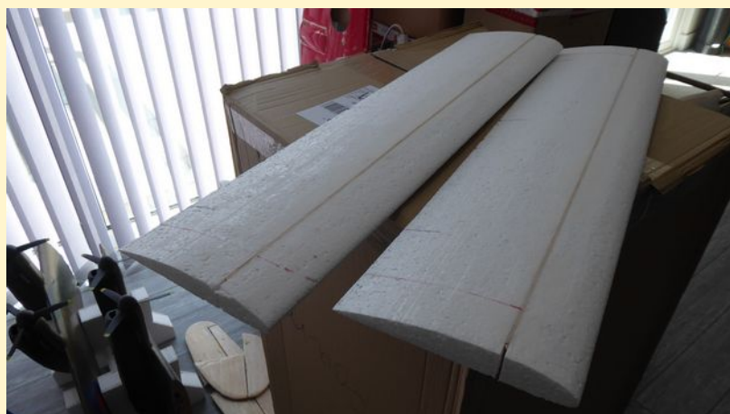
Wing cores with spar in place
