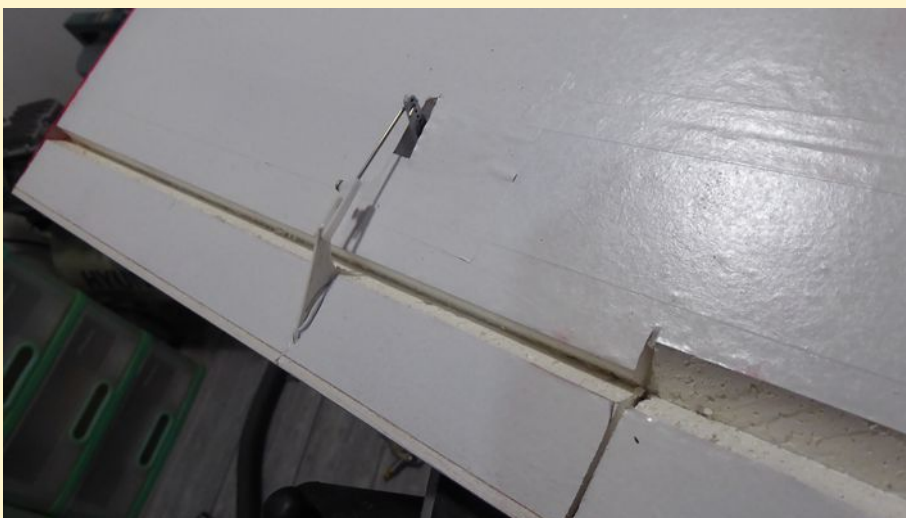
Hinge cuts and servo fitment
