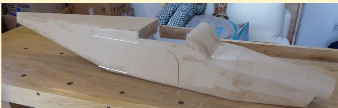
Completed fuselage covered with brown paper
