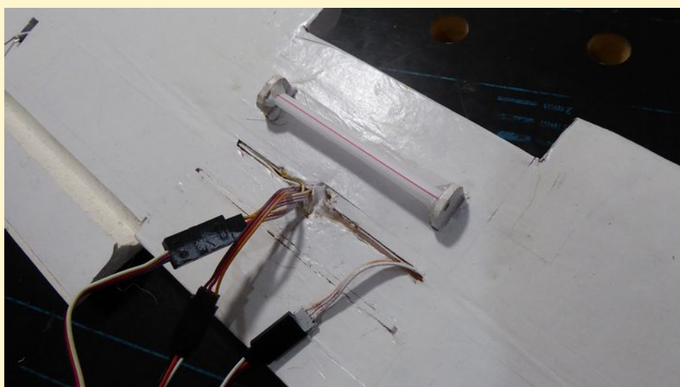
Wing centre showing tabs with guide straw
