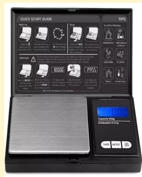
A cheap digital scale enables accurate ratios of adhesive and hardener
