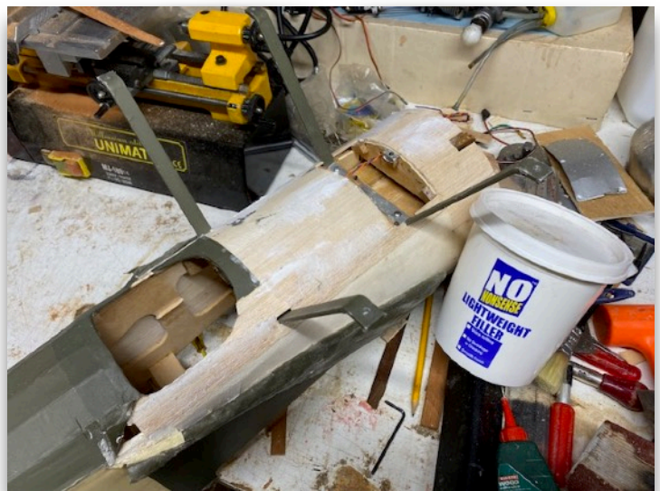
Picture 17 shows the fuselage skinned and nearing completion.
