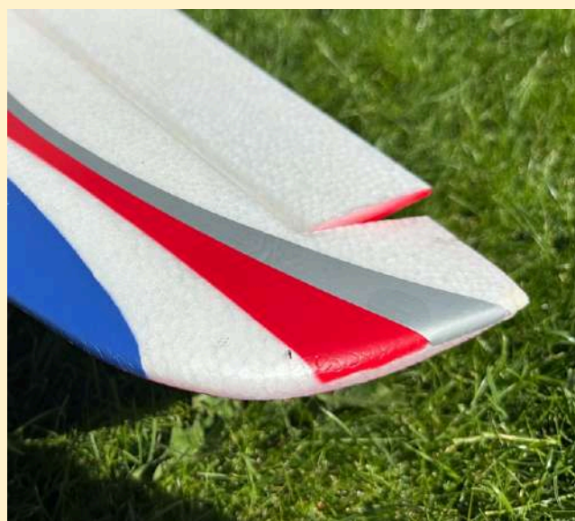
Full “Up” Elevator for Mid Rates (loops etc.)!
