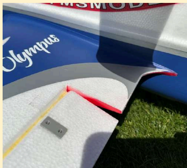
Full Aileron movement for Low Rates (rolls)
