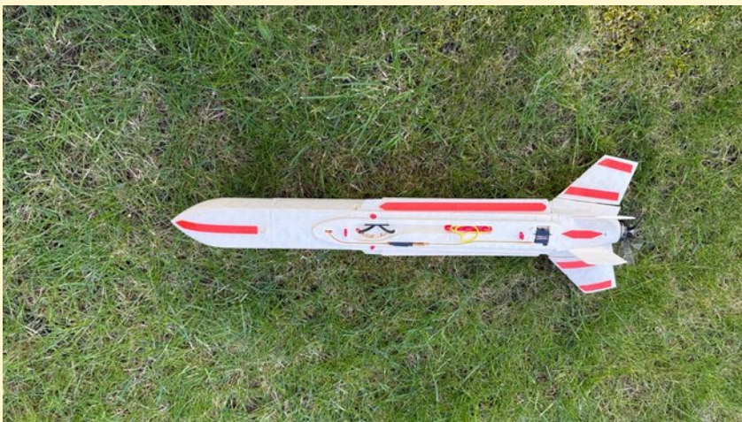
Micro-cruiser with wings folded inside fuselage body. The missile and wing release mechanism is just visible on top of the model. Non-ducted fan power plant at the blunt end
