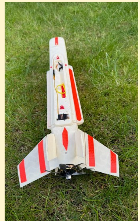
Blunt end showing non-ducted fan and elevon control surfaces
